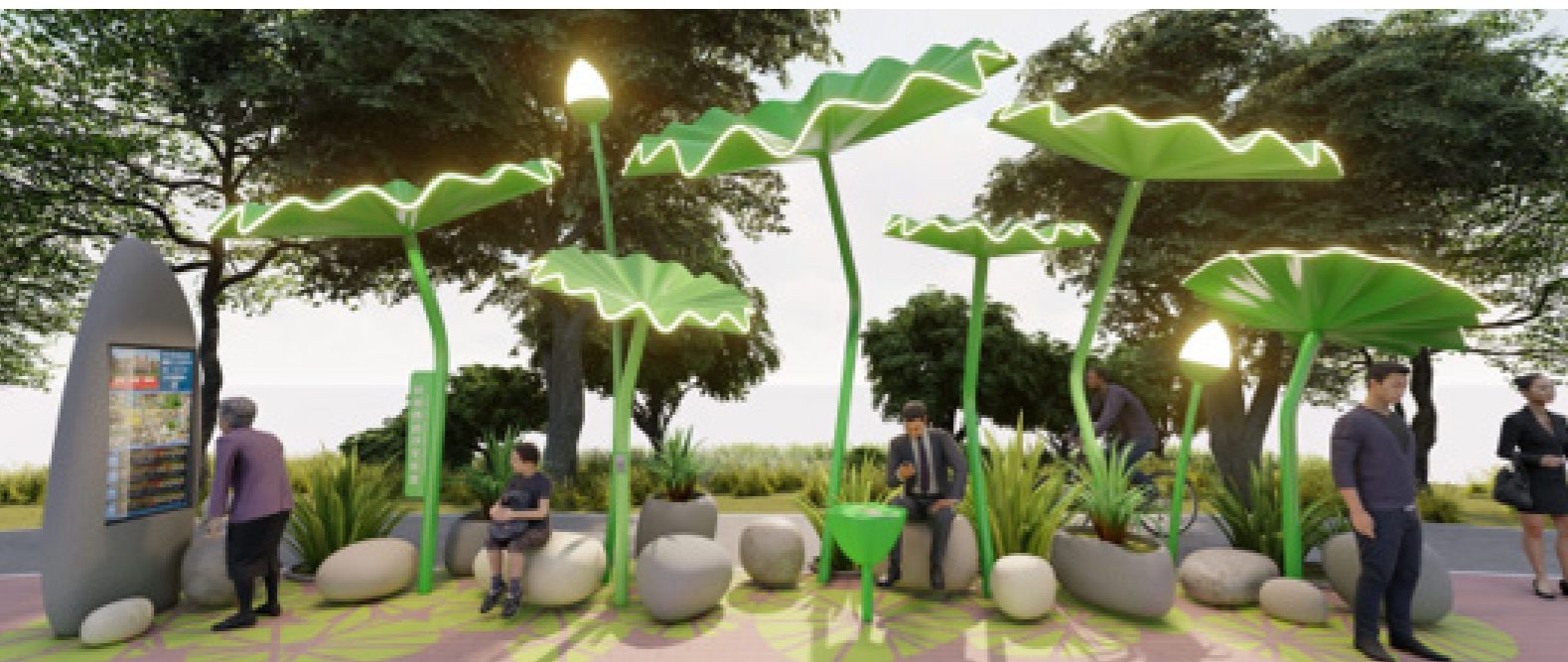
A potential structural implementation of a mobility station of the future with various features, such as solar systems for power generation, WiFi hotspot, seating and roofing. In the future, different modes of transport (such as public transport, cars, bicycles, scooters) will come together in these stations in order to make it easier to switch from one mode of transport to the other.
